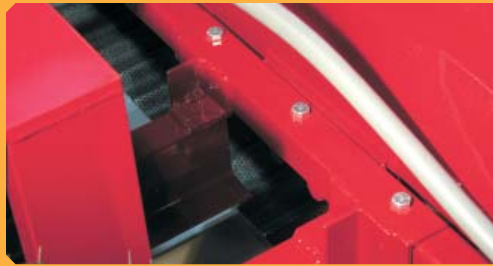
Tractor Frame Bolted to Sweep Assembly.
